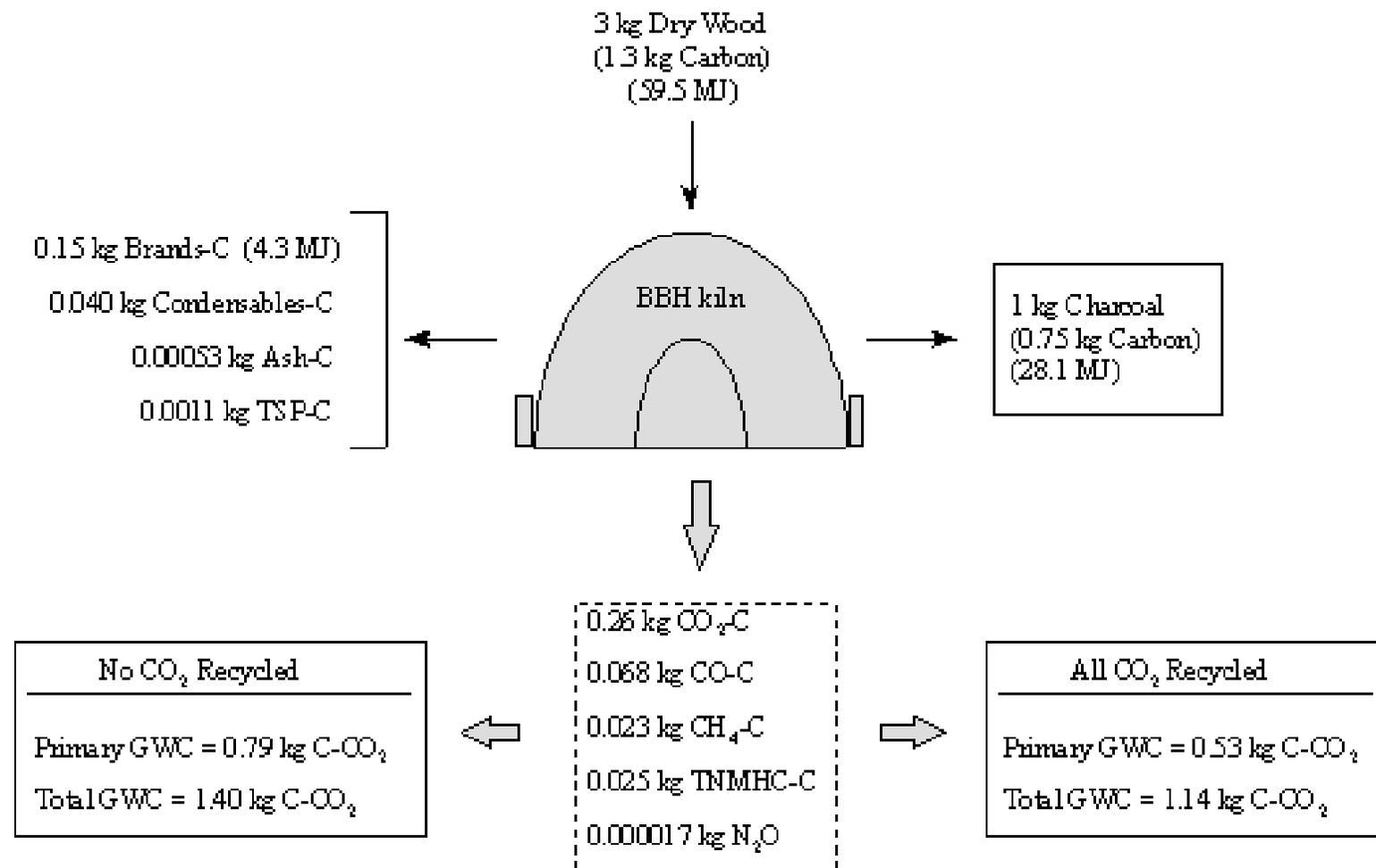
Figure 1. Carbon cycle for charcoal making in the BBH kiln and the GWC resulting from renewable and non-renewable harvesting of the wood. GWC = Global Warming Commitment in kg C as CO<sub>2</sub> equivalent.
