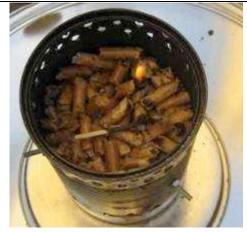
A common 425-ml tin-can served as fuel chamber, which was filled to a level of 70 mm with 200 g of standard 6-mm pinewood pellets. A 10-mm layer of pellets soaked in paraffin (kerosene, lamp-oil) was spread out evenly on top as lighting material and lit from the top with a match to initiate the pyrolysis process of the pellets in the fuel chamber.
