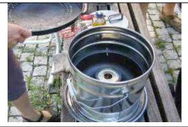
In this demonstration the flame of the afterburner was established already well enough after 2 minutes, to accommodate the skillet, a modified pizza-tray, on top.
